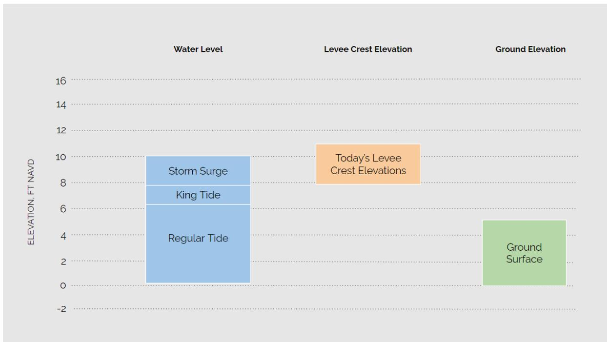
**Figure 5.** Ranges of water surface elevations, ground surface elevations of diked baylands, and levee crest elevations in the diked baylands on the eastern side of the Petaluma River. Elevation data from Buffington and Thorne (2019).
